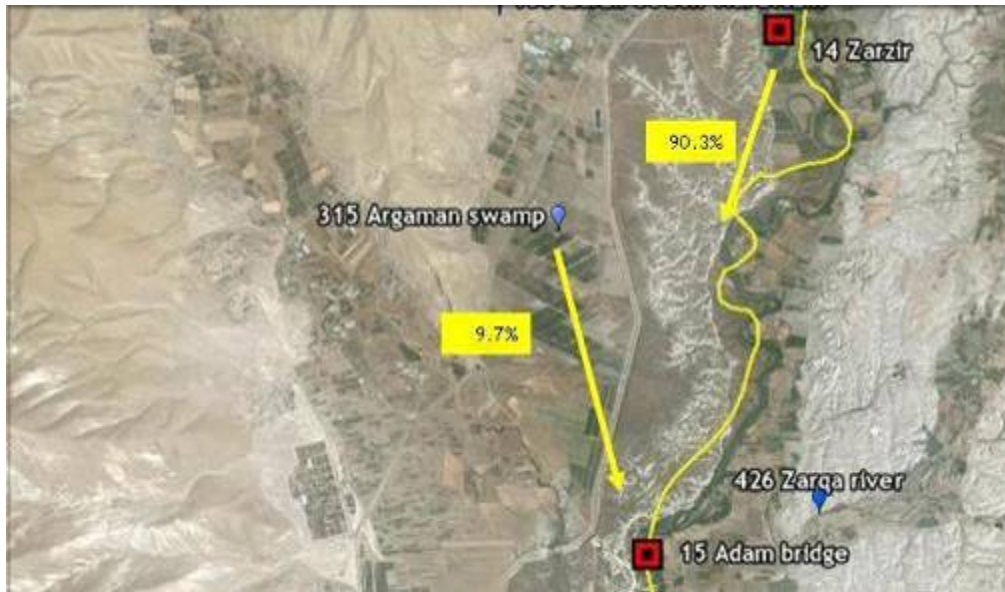
Figure 21: Sources of water contributing to the flux of the Jordan River at Adam Bridge (Cell 15), summer 2001.
