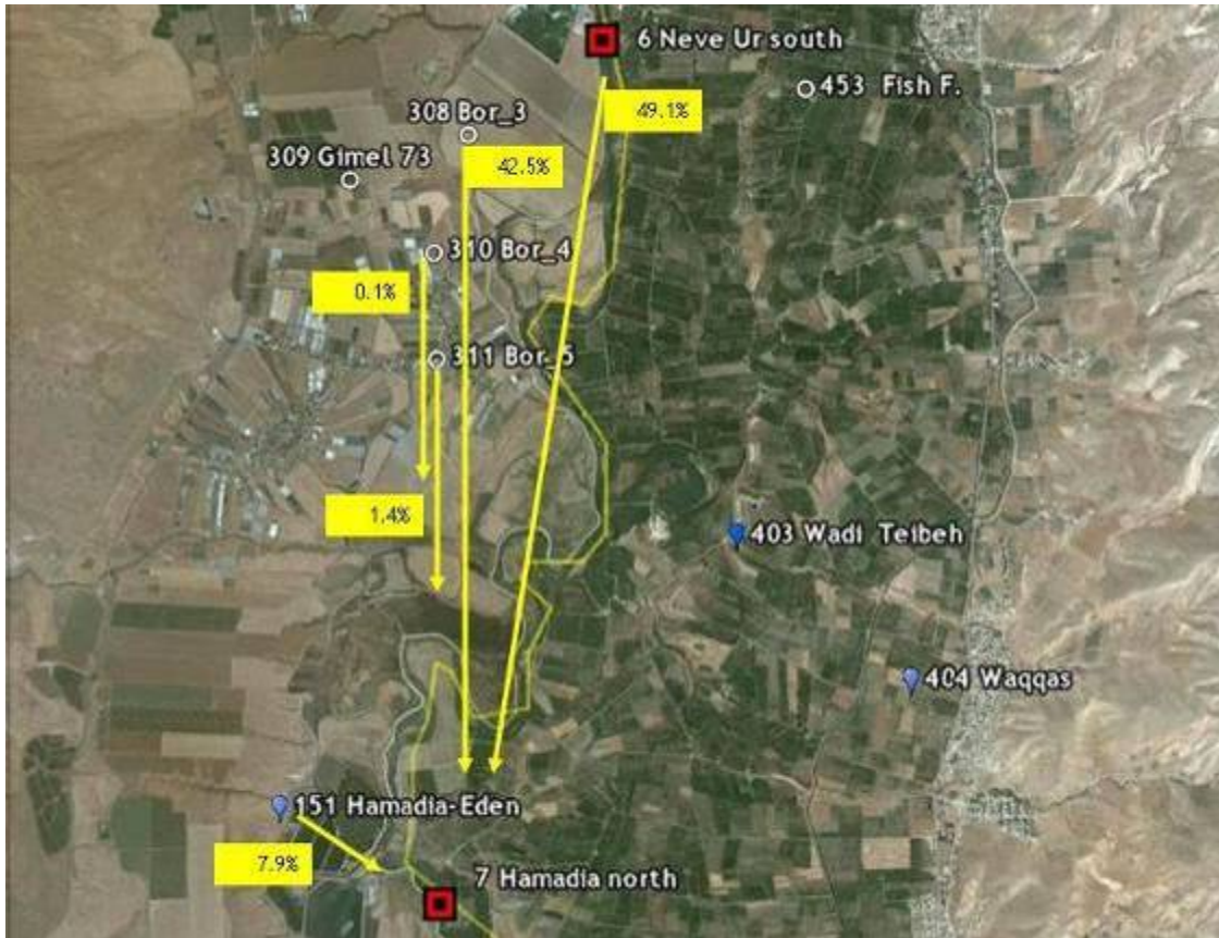
Figure 14: Sources of water contributing to the flux of the Jordan River at Hamadiya North (Cell 7), summer 2001.
