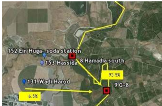
Figure 16: Sources of water contributing to the flux of the Jordan River at NeMaoz Haim (Cell 10), winter 2001 fluxes.
